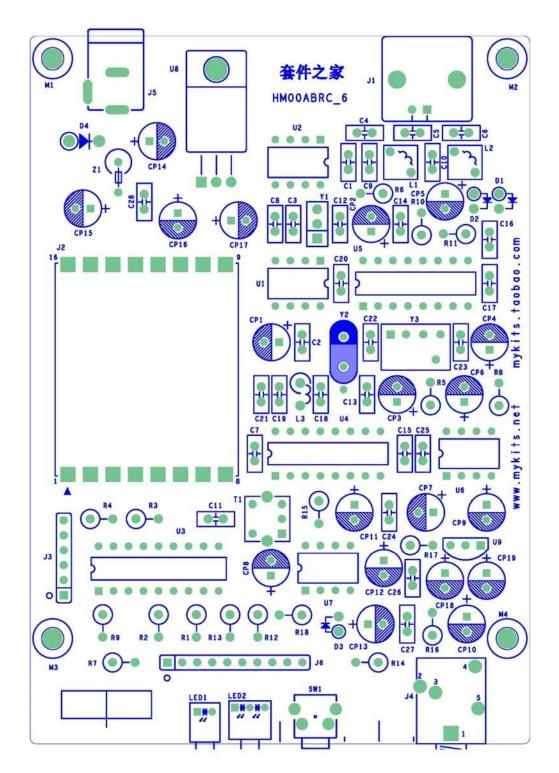
Please note pin 1 of Y1 (10.7MHz ceramic filter). It must be installed in the correct direction!
