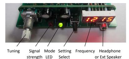
From left to right, the knobs and buttons of this machine are: tuning knob, signal received LED (signal strength indicator), Mode indicator LED, Mode selection button, and the headphone jack.
