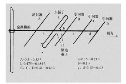
The metal mast should be at the rear of the Yagi antenna. This ensures the mast will not have a significant impact on the antenna radiation field. In the diagram,  $\lambda$  is the wavelength. The antenna can be assembled after calculating the length of the director, the reflector and the other antenna elements, and the spacing a, b, c, and d.
