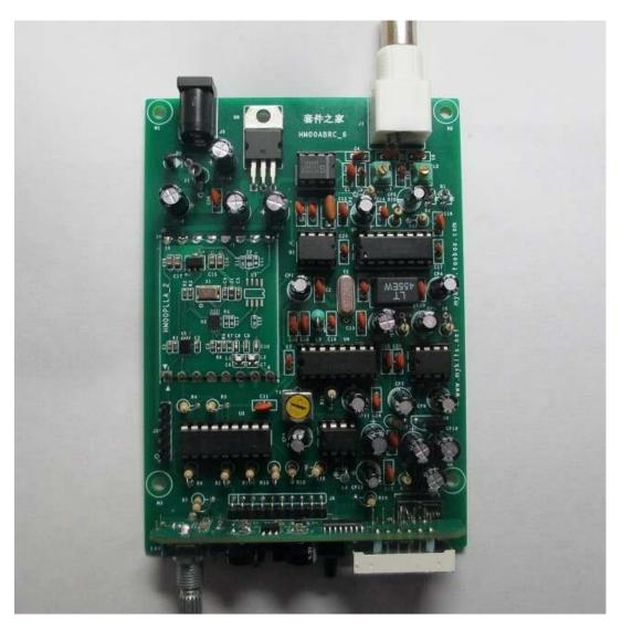
The hardware described in this article is V6.0 and the PCB labelled "HM00ABRC\_6"
